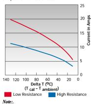
Delta T is the difference between the zero current calibrated opening temperature ( $T_{cal}$ ) and ambient temperature ( $T_{ambient}$ ) at the protector location.
